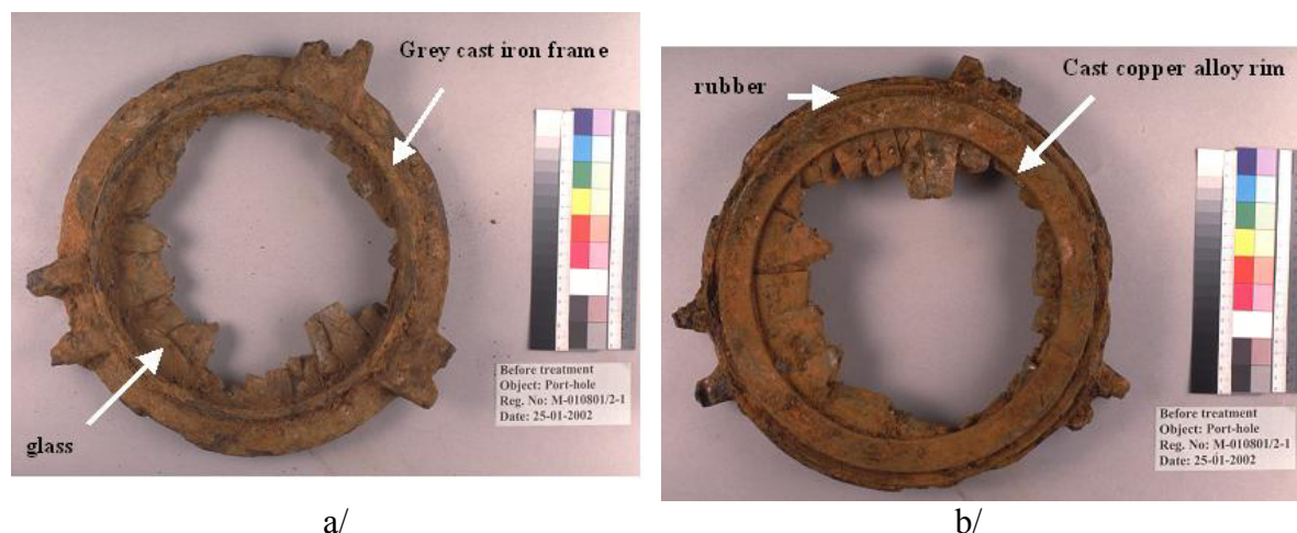
Figure 1: General view of the porthole (a/ front side and b/ rear)
