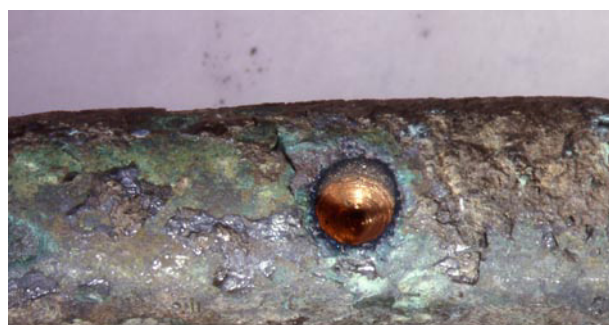
Figure 4: ‘Black spots’ forming along a tear in a Roman bronze fibula (A 584 a) 5 .
