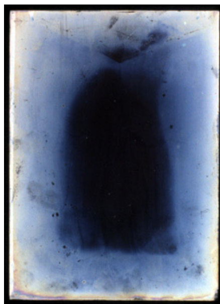
Figure 1 Silver gelatine glass negative with wide silver mirroring stain, partially obscuring the image. Cueni study collection (~1910).
