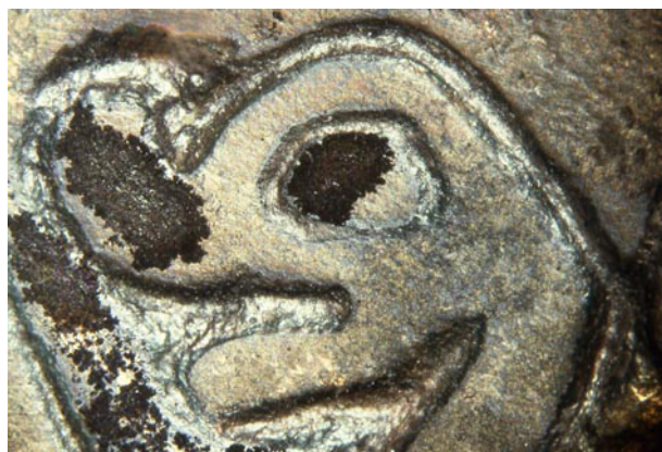
Figure 7: ‘Black spots’ covering large parts of a medieval bronze fibula (KN 116) 8
