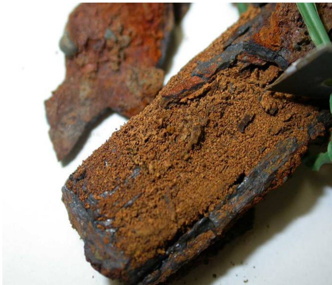
Figure 3 Akaganeite growing on iron substrate
