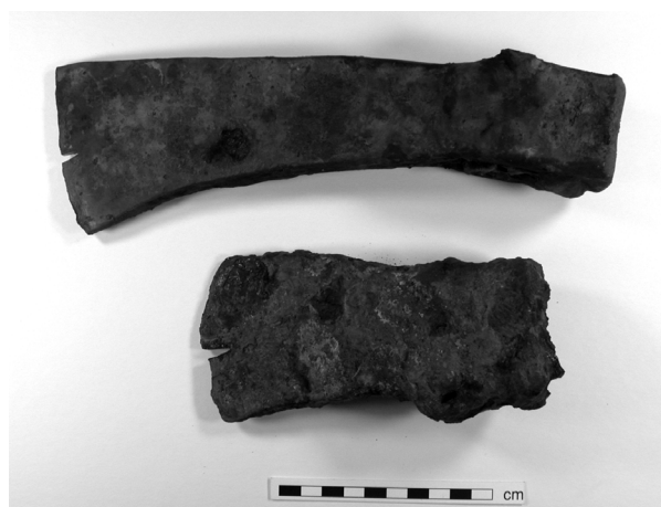
Figure 1. Axeheads 11 (upper) and 131 from Fiskerton excavations 2001. The lower axehead (131) is socketed and lugged. The ‘V’ notches from the cutting edges (left) are where the metallographic samples have been removed.
