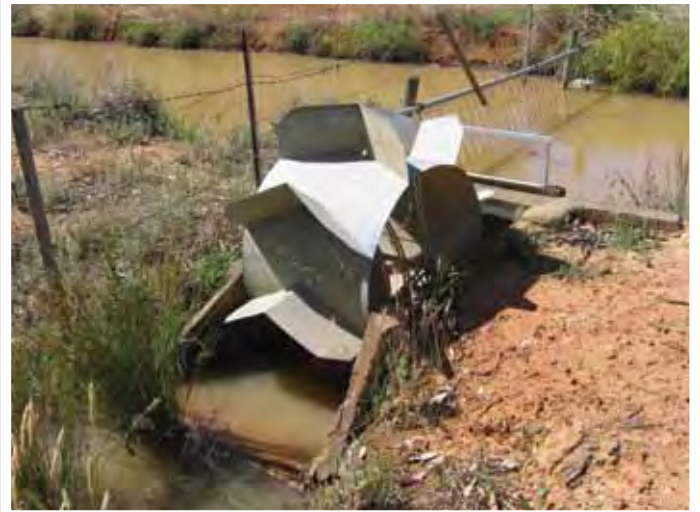
The Dethridge water meter wheel has been produced in thousands and is a symbol of Australian irrigation
