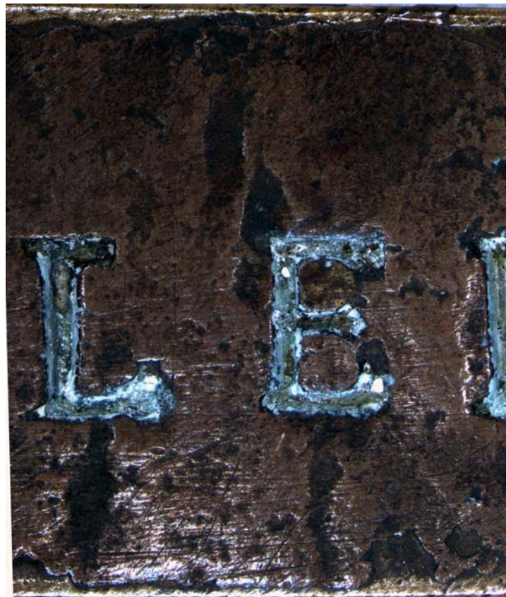
Figure 14: Photographic image of the letters “LEI” showing presence of the white titanium based pigment inside the lettering, where the original black shellac has been lost.
