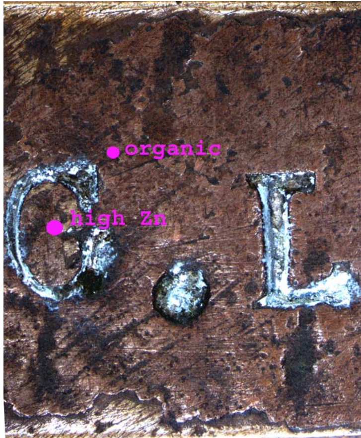
Figure 11: Optical image of the plaque at the separation of LUDWIG•LEICHHARDT showing overlapping layers of metal near the foot of the image and areas shown in the SEM Figure 12.
