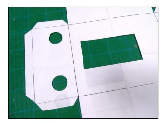
**Step 2:** Lay the six template sheets out on a large sheet of card, in two rows, matching the numbers 1–4. Glue into place. **Step 3:** Ask an adult to cut around the template, using a utility knife on a cutting mat. Cut out the shaded rectangle and circles. **Step 4:** Test your cardboard tubes in the circles and adjust to fit.
