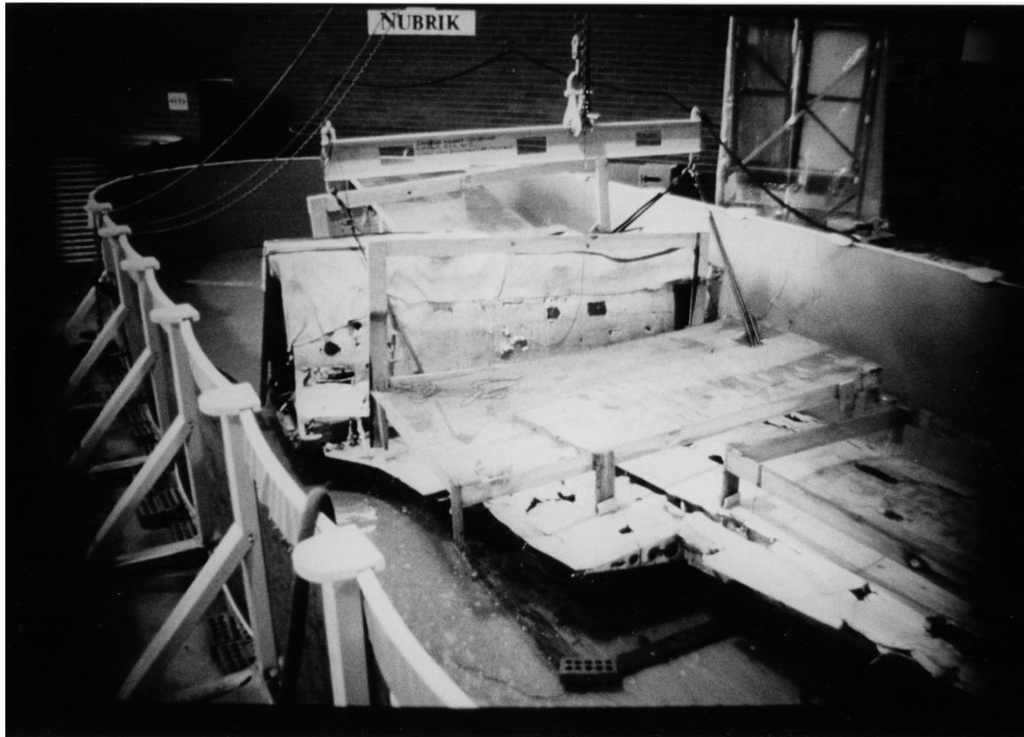
Figure 2. Oscar wing and cockpit section in the pool to check the position of the bottom anodes.
