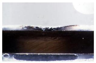
Figure 8: Copper test plate coated with microcrystalline wax COSMOLLOID H80<sup>®</sup>; a black, sulphurous corrosion had grown through a pore in the coating after exposure at ca. 4 ppm hydrogen sulphide for several weeks. A slight depression in the metal surface is visible<sup>9</sup>.
