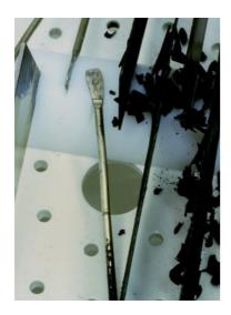
sulphide. The corrosion started to spread to the pewter, from a point where the two plates touched (Figure 9). The corrosion spread over a distance of approximately 3 cm.
