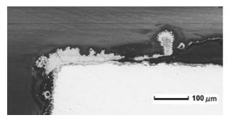
Figure 11: Copper test plate coated with microcrystalline wax (COSMOLLOID H80<sup>©</sup>, appearing black); 'black spots' grow along the edge, where the protective coating is thinned (application by immersion). The sample was exposed to hydrogen sulphide concentrations of ca. 4 ppm for three months<sup>12</sup>.
