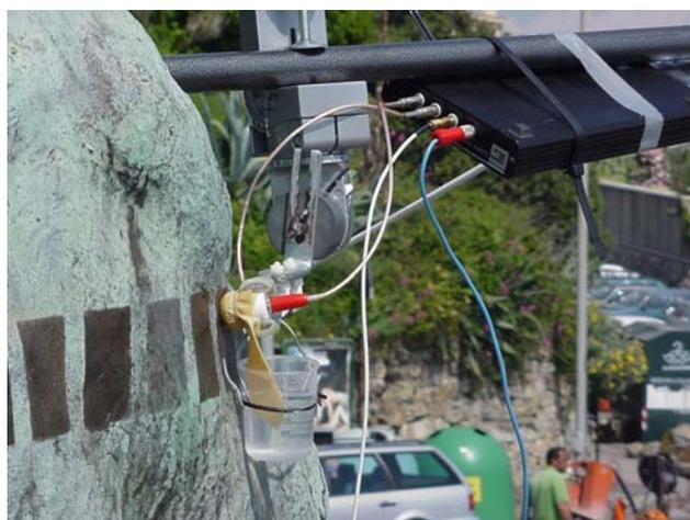
Figure 1 Electrochemical Impedance Spectroscopy measurement with the contact probe on *Monumento ai Mille* (test area III). From left to right, the visible 6x4.5 cm test zones are the ones for [B], [C], no coating, [E], and [F].
