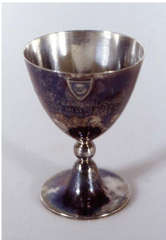
Figure 10. Silver chalice (LM 79223) prior to hydrogen plasma reduction with disfiguring tarnish layer.
