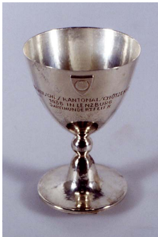
Figure 11. Silver chalice after 2.5 hours of hydrogen plasma reduction, no other surface treatment has been applied.
