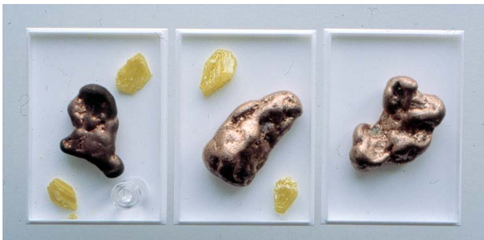
Figure 1 Copper nuggets, stored with sulphur crystals (middle), additional water (=100 % rH, left) and blank experiment (no sulphur, right) in polystyrene boxes, after one year.
