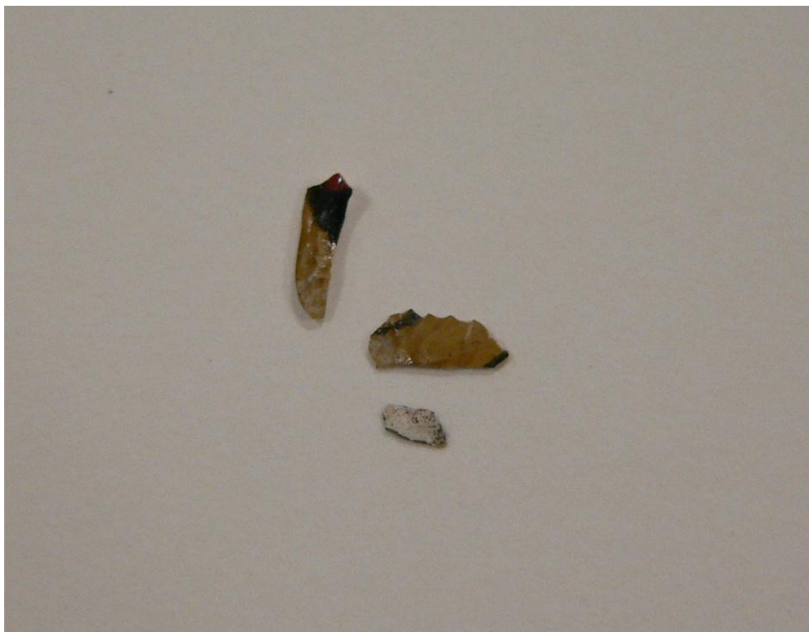
Figure 2 – Fragments of dislodged paint
