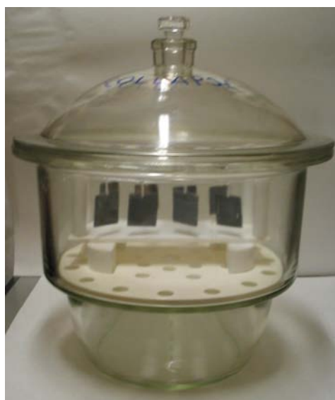
Figure 1 Accelerated corrosion test equipment.
