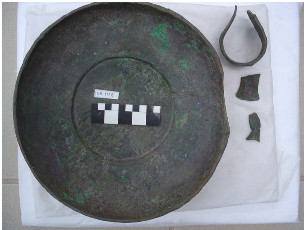
Figure 5: CA-108 after the treatment with BTA and AMT.
