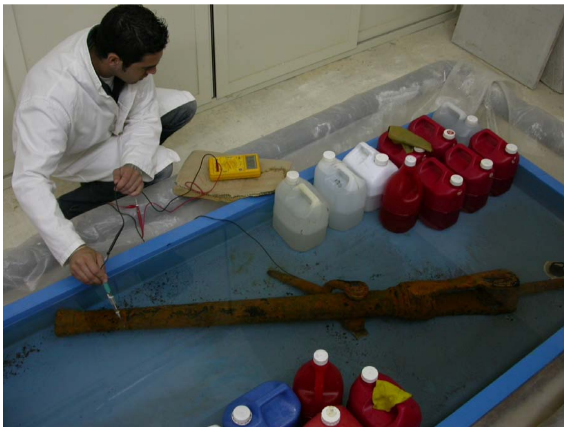
Figure 13: Principle of the measurement of E_{\text{corr}} with a reference electrode. The artefact is an iron based swivel gun immersed in 1% NaOH solution (credit: D. Vella)
